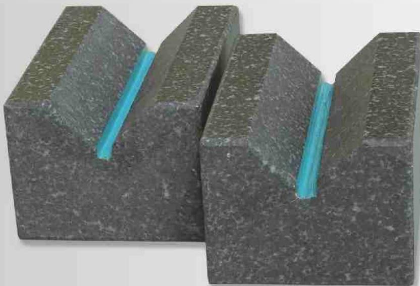
*High precision V-blocks made from black granite and suitable for checking cylinders. The tolerances given in the table refer to planarity of the base, and to parallelism between the base and the 90° "V"s axis. Supplied in pairs.*
