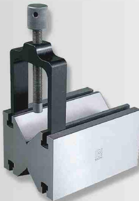
*Prism with clamp made from hardened, stabilised stainless steel. Entirely ground. With two 90° "V"s. Manufactured to tolerances of planarity and parallelism  $\leq 0,005$  mm. Supplied singly.*
