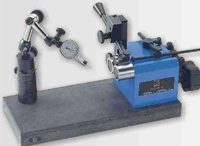
**Instrument for concentricity and perpendicularity control.** Robust and compact design for laboratory and workshop use. Easy and precise for measuring and control. Adjustable rollers and clamping pressure. Transmission through a gear belt. Adjustable dial stand on 360°. Accuracy of roller 2 µm. Using thread rollers, the concentricity in reference to the threads can be verified. Supplied without dial test indicator.
