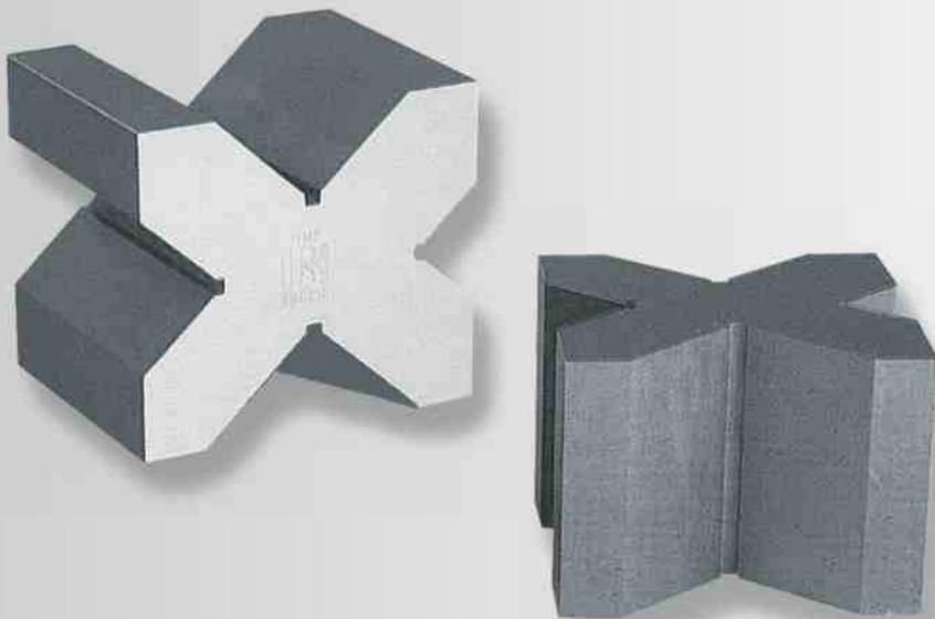
*High precision V-blocks. Made from hardened, stabilised stainless steel. Entirely ground. With four 90° "V"s. Manufactured to tolerances of planarity and parallelism  $\leq 0,005$  mm. Supplied in pairs.*
